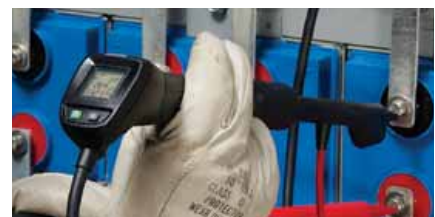
BT521 Intelligent Test Probes with integrated display
